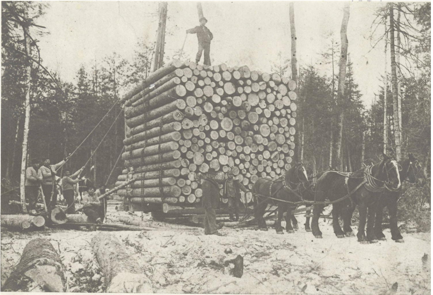
18569 c. 1916 "Star Load" at Rib Lake Lumber Co. Camp 9 in Price County. With assistance from steam hauler, horses pulled sleigh on ice road to Rib Lake.
